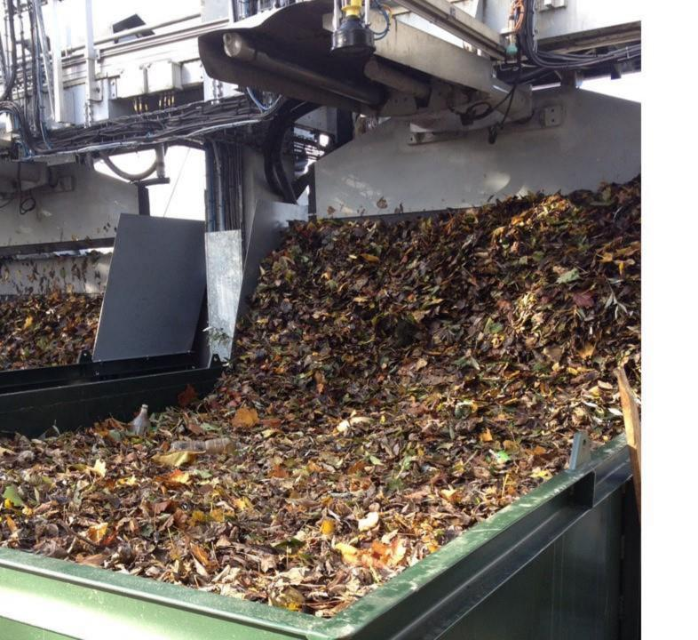
River waste is mixed up steadily thanks to a double moving floor and dries quickly.
