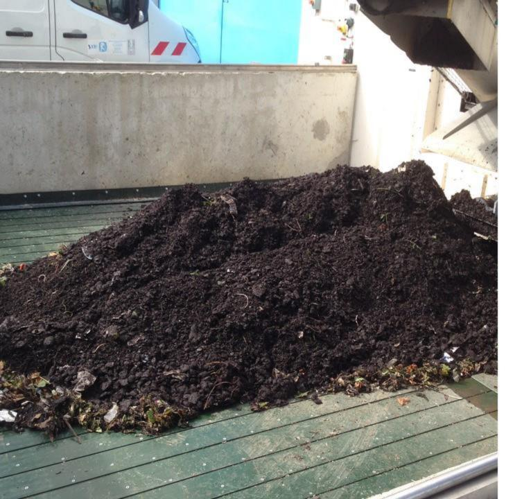
Organic residues of a screen are spread on a large moving floor.
