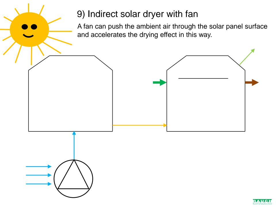
Radial fans "pumping" the heated ambient air into the dryer
